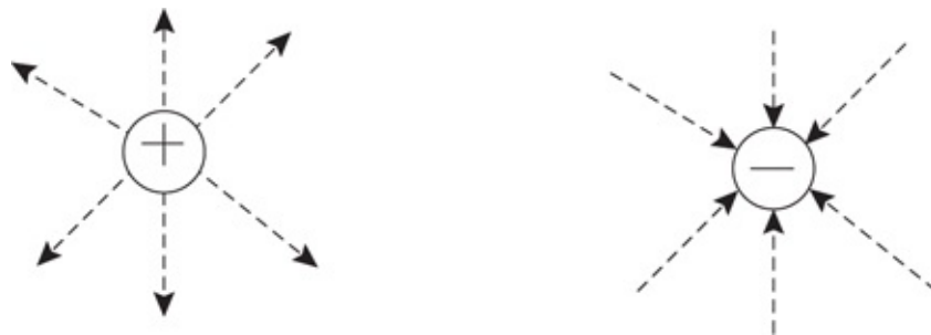
Figure 18.5 Electric field produced by point charges.
