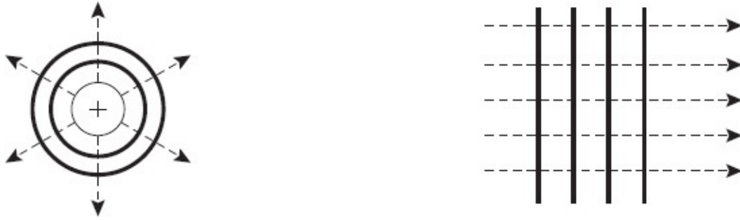
Figure 18.2 Two examples of equipotential lines (in bold) and electric field lines (dotted).
