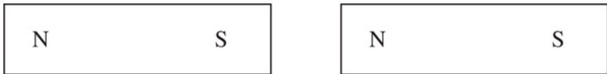
Figure 20.2 Cutting the bar magnet in Figure 20.1 in half just gives you two smaller bar magnets. You can never get an isolated north or south pole.
